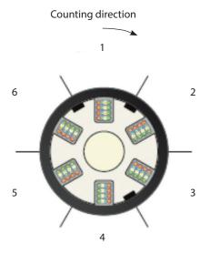
Slotted Core Profile, 8-fiber Ribbon, 8 to 192 Fibers
