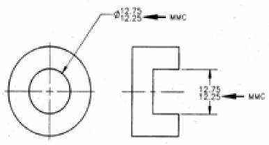
Example 1-9. Maximum Material Condition (MMC) for internal features.
