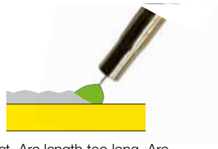
Incorrect. Arc length too long. Arc becomes too wide, giving insufficient penetration and a risk of slag traps. Also a risk of burnback to the contact tip. This may be caused by the arc voltage being too high, the wire feed speed too low or the stick-out being too short.
