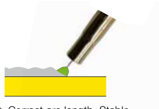
Correct. Correct arc length. Stable and concentrated arc with a quiet spray droplet transfer.
