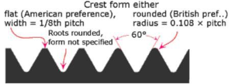
In the compromise the British accepted the 60° thread angle, and the Americans accepted rounded roots and optionally rounded crests. Five classes of fit were defined. The new fasteners continued to fit, for most practical purposes, ones manufactured under the old American National Standards. NC became UNC, NF became UNF, etc.
